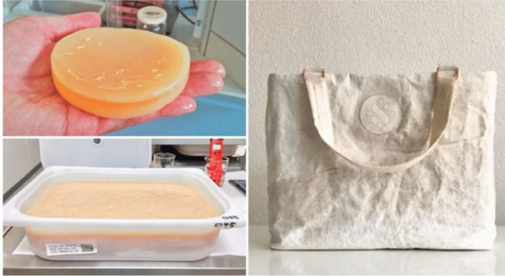
Unprocessed bacterial cellulose is a bit like wet leather. When dried, it can be made into products like handbags. Source: Choi M.S., et al./Polymers, 2022
